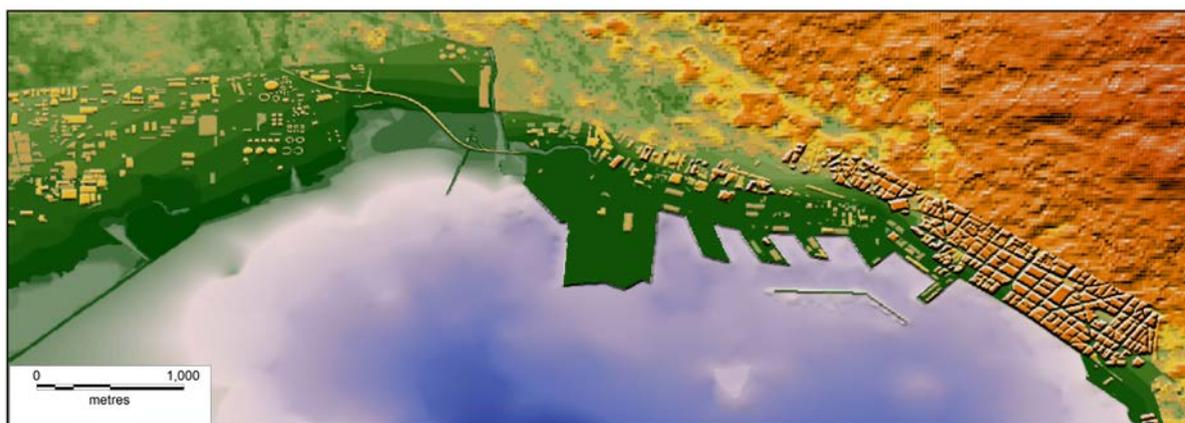
Figure 61 : Snapshot of the high resolution grid (10 m) of the Thessaloniki bay area. This grid will be used to perform simulations of inundation.
