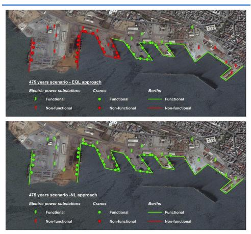
Functionality of components in the harbour application for an earthquake scenario with 475 years return period, for equivalent linear (top) and nonlinear analysis approach (bottom)
