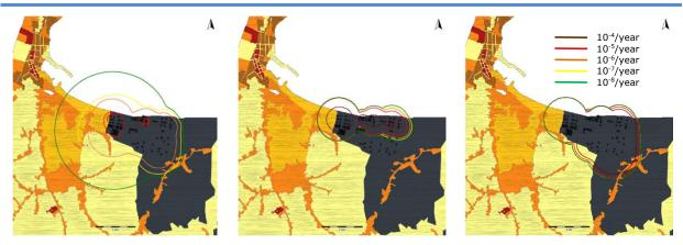
Risk contours for industrial (a), tsunami (b) and earthquake (c) risk in the petrochemical plant
