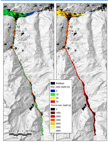
Inundation resulting from overtopping of the conceptual-dam application
