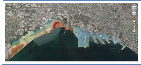
Site-specific tsunami inundation modelling results on a high resolution grid of the application in the port of Thessaloniki
