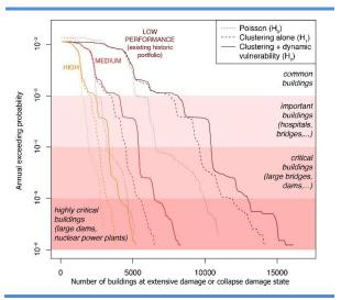
Seismic risk curves in a conceptual example in northern Italy, with amplification of risk due to the combination of earthquake clustering and damagedependent vulnerability of buildings
