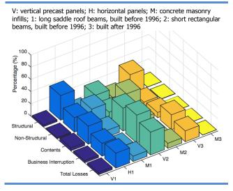
Disaggregation of average annual loss in the industrial district application, according to building sub-class for each component of loss
