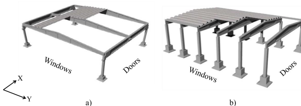
Fig. 5.1 Structural configuration of Italian precast warehouses
