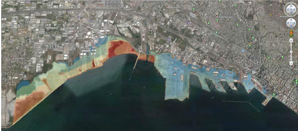
Fig. 3.3 Site-specific tsunami inundation modelling results on a high-resolution grid of the application in the port of Thessaloniki (Selva et al 2016; Pitilakis et al 2016)
