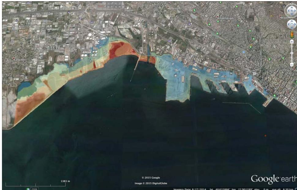
Figure 62 :Example of tsunami inundation modelling results on a high resolution grid
