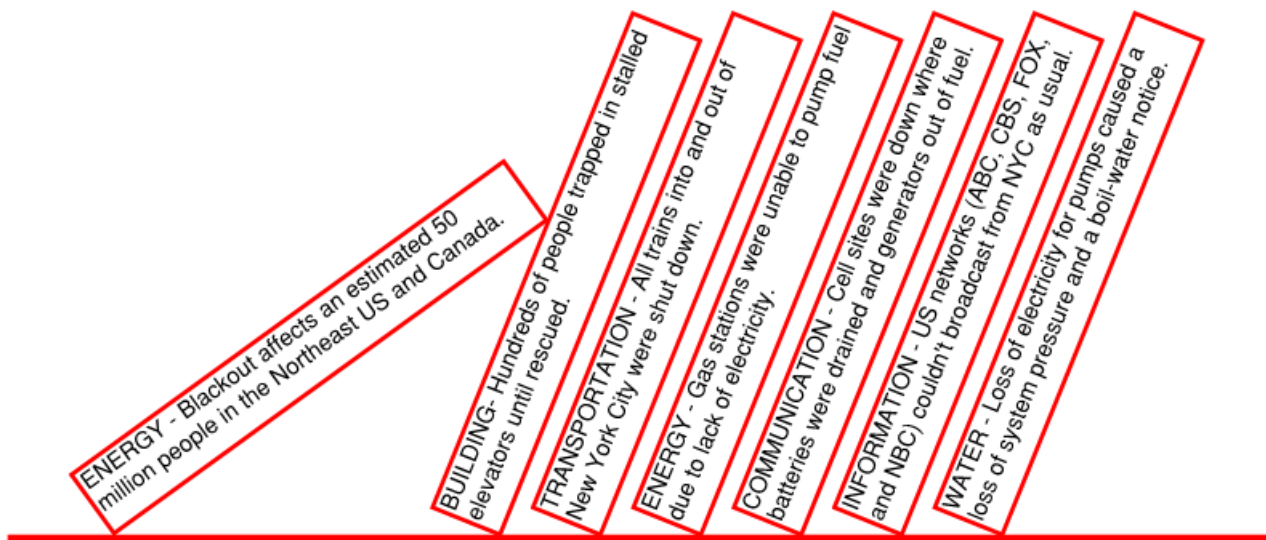
Fig. 6.19 Inter-dependence cascading failure in the 2003 Northeast blackout (NIST, 2015).
