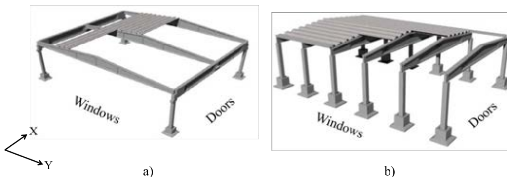
Figure 5.4: Structural configuration (Casotto et al. 2015) and assumed position of openings in a) Type 1 buildings and b) Type 2 buildings
