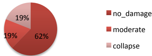
Figure 6 Distribution of damage for the buildings in the exposure model
